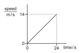
Which calculation gives the distance travelled by the car in 24 seconds?
