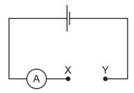
Four wires of different length and thickness are connected in turn between point X and point Y. All four wires are made of the same metal.
